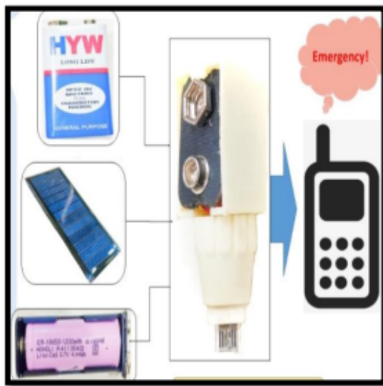
Figure 1.2: EPB with Multiple power sources.
